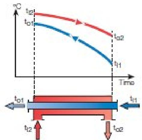
Fig 6.1.7 Temperature profiles for heat transfer in a heat exchanger
