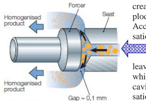
Fig. 6.3.2 At homogenisation, the milk is forced through a narrow gap where the fat globules are split.
